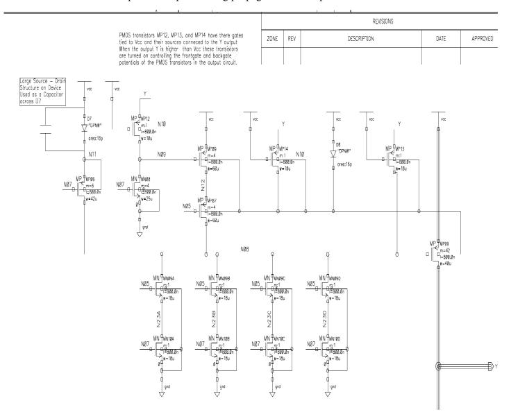
4. The merged transistors MN9 and MN10 are denoted below. This discharges the gate and turns on the large PMOS output. Node 8 is connected to Y during the Ioff Condition
