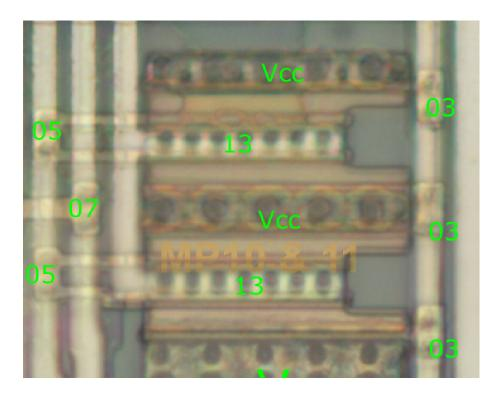
3.The Ioff circuitry. A key feature of the LVC family is to allow a high voltage to be applied to the output while Vcc=0V and have only a very small leakage current to flow.
